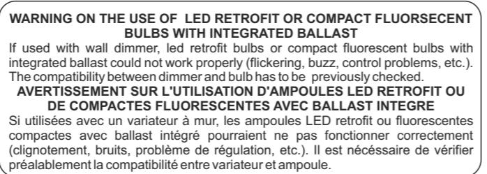
**WARNING ON THE USE OF LED RETROFIT OR COMPACT FLUORESCENT BULBS WITH INTEGRATED BALLAST**
