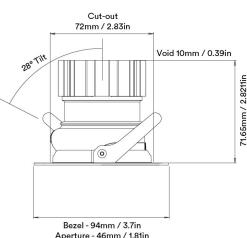
Unit height increases by 21.65mm / 0.85in for spot and elliptical beams
