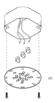
Note: Make sure the supplied Universal Mounting Plate is fastened directly to the junction box. The surface of the junction box should be set back 1/8" or 3mm from the mounting surface. This will ensure the best possible fit for ease of installation and final finish. Note below the correct and incorrect fit for optimum installation.
