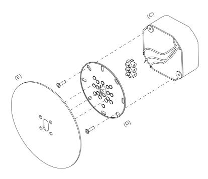
Note: Make sure the supplied Universal Mounting Plate is fastened directly to the junction box. The surface of the junction box should be set back 1/8" or 3mm from the mounting surface. This will ensure the best possible fit for ease of installation and final finish. Note below the correct and incorrect fit for optimum installation.
