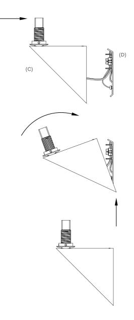
Screw the grub screw (A) using the allen key provided (B) in order to secure the main body (C) to the backplate (D).
