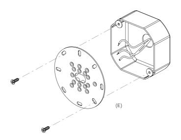
Note - Make sure the supplied Universal Mounting Plate is fastened directly to the junction box. The surface of the junction box should be set back 1/8" or 3mm from the mounting surface. This will ensure the best possible fit for ease of installation and final finish. Note below the correct and incorrect fit for optimum installation.
