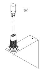
Screw the opaline glass (I) onto the lamp holder.
