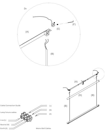
Secure the ceiling rose (D) to the back plate (A), using 4 grub screws and allen key (F) provided, making sure no cables are sticking out during this procedure.
