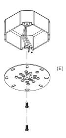
Note - Make sure the supplied Universal Mounting Plate is fastened directly to the junction box. The surface of the junction box should be set back 1/8" or 3mm from the mounting surface. This will ensure the best possible fit for ease of installation and final finish. Note below the correct and incorrect fit for optimum installation.
