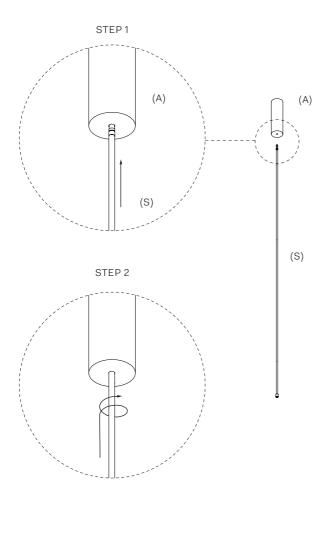
Note: The illustration below is only for extra length in the pendant rod. It shows the joint connection between the two pendant rods.
