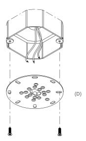
Note: Make sure the supplied Universal Mounting Plate is fastened directly to the junction box. The surface of the junction box should be set back 1/8" or 3mm from the mounting surface. This will ensure the best possible fit for ease of installation and final finish. Note below the correct and incorrect fit for optimum installation.
