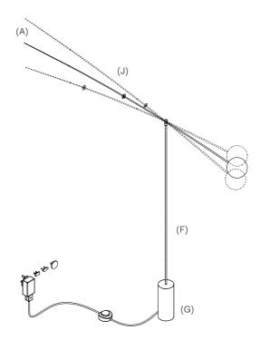
Note: Do NOT lift the light from the Lamp body 1 (F) but from the Floor Base (G).
