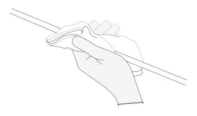
On a soft surface, using gloves, secure the Spike (A) onto the Lamp Body 2 (B).
