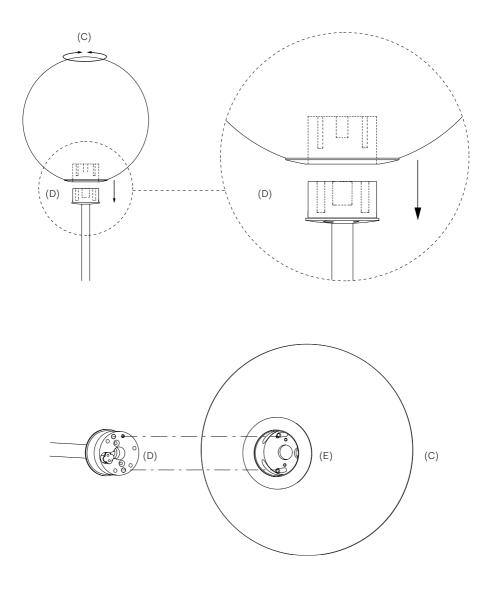
Secure the Large Glass Sphere 1 (C) with the supplied M2×20 screw and hex key, ensuring it is tight to keep the connectors flush.
