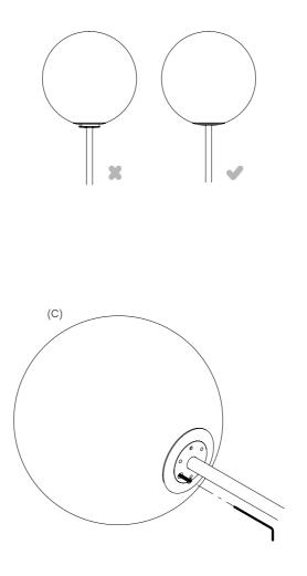
Using gloves, carefully insert the Lamp Body 1 (F) into the Floor Base (G). Whilst applying downward pressure, gently turn the Lamp Body 1 (F) clockwise until you feel a small click. This is the 'clutch' engaging. It will feel like it has locked, but keep gently twisting until you cannot twist any further and carefully release the Lamp Body 1 (F).
