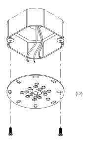
Note: Make sure the supplied Universal Mounting Plate is fastened directly to the junction box. The surface of the junction box should be set back 1/8" or 3mm from the mounting surface. This will ensure the best possible fit for ease of installation and final finish. Note below the correct and incorrect fit for optimum installation.
