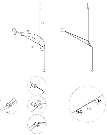
Each joint has a free 360 rotation, allowing the Mobile Chandelier to be positioned according to the space. Lamp Body 1 (L) can rotate freely about the Pendant Rod (Q).
