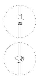
Using gloves, support the Lamp Body 1 (L) and carefully insert the Joint Boss (R) into the Pendant Rod Cap (S). Gently screw them together until tight. Then screw the Lamp Body 2 (P) onto the Lamp Body 1 (L).
