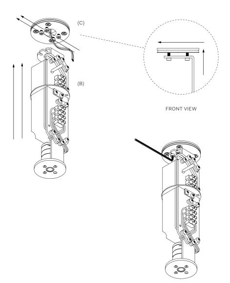
Carefully pull the supply wires ensuring there is no excess wire. Secure them using the Wire Grip (G), leaving enough wire to be able to reach the Terminal Block (H).
