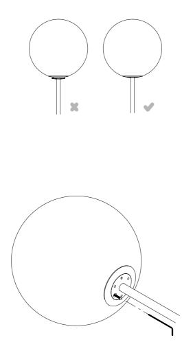
On a soft surface, using gloves, screw the Brass Sphere Weight (O) onto the Lamp Body 2 (P).
