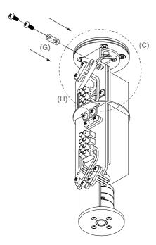
Connect the live, neutral and earth of the mains electrical cable to the terminal block of the fixture. Make sure all electrical cables match correctly.
