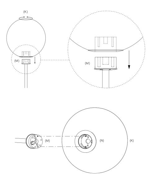
Secure the Large Glass Sphere 1 (K) with the supplied M2×20 screw and hex key, ensuring it is tight to keep the connectors flush.
