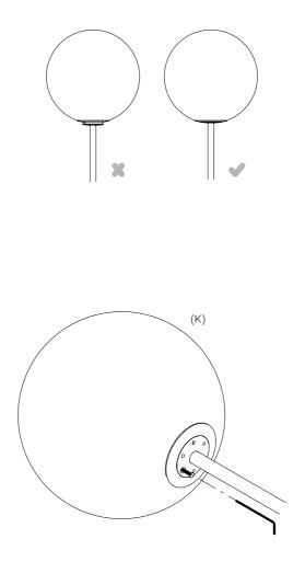
Carefully rotate the Large Glass Sphere 1 (O) onto the Small Male Glass Connector (Q1) until the internal location pins are aligned. Gently push the Large Glass Sphere 1 (O) onto the pins until the outside faces of the Small Female Glass Connector (Q2) and Small Male Glass Connector (Q1) sit flush.
