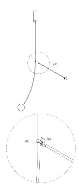
Each joint has a free 360 rotation, allowing the Mobile Chandelier to be positioned according to the space. Lamp Body 1 (L) can rotate freely.
