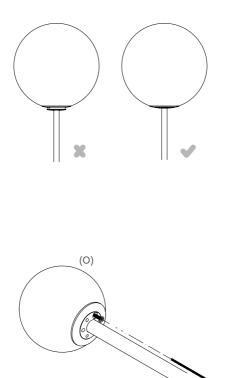
Using gloves, carefully insert the Lamp Body 1 (L) into the Ceiling Rose (A). Whilst applying upward pressure, gently turn the Lamp Body 1 (L) clockwise until you feel a small click. This is the clutch engaging. It will feel as if the Lamp Body 1 (L) has locked but keep gently twisting until it will not twist any further then carefully release the Lamp Body 1 (L). It will feel like it drops slightly. This is the clutch disengaging and the Pendant Rod will now rotate freely.
