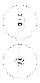
Using gloves, support the Lamp Body 2 (P) and carefully insert the Joint Boss (R) into the Lamp Body 2 Cap (S). Gently thread screw them together until tight.
