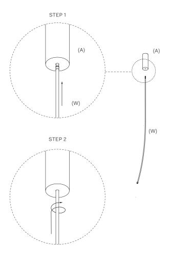
Note: The illustration below is only for extra length in the pendant rod. It shows the joint connection between the two pendant rods.
