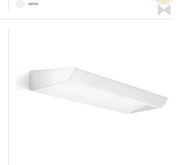
Wall lighting fixture for interiors, with direct and indirect light emission. Pickled sheet metal wall bracket in polyacrylic paint. Extruded aluminium structure in white, black, bronze, mat brass or titanium polyacrylic paint. Extruded acrylic diffusers with opaline finish.
