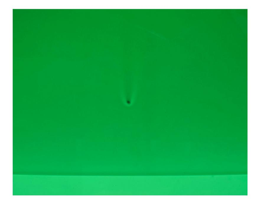
During the procedure of dipping the shade in paint, the lamp can take on various markings such as lines, lumps or the opposite, small bubbles that prevent the paint from building up and allowing the opal glass to show through.
