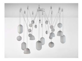
**Tech. description** The light is hung from a central metal ceiling canopy, which houses the electronics and anchors the wire ropes integrated into the power cables leading to each light. The individual lights are hung from the ceiling by means of pulleys and balanced with counterweights. The system allows variable vertical positioning of each light independently. Each light comprises a power cable, metal cover, LED module, and a glass shade.
