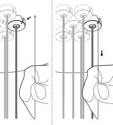
Very carefully uncoil the braided coaxial cable in a spool like manner. Insert your index fingers into opposite sides of the roll then rotate your fingers around each other to unroll the coaxial cable.
