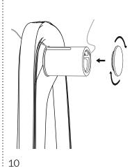
Screw frame cap back onto the frame assembly.
