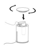
Screw cap back onto the lamp holder assembly.
