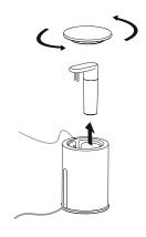
Unscrew cap at the aircraft cable end of the : Remove lamp from lamp adapter and lamp holder assembly. Push coaxial cable through the slot in the silicone sheath, and remove lamp and lamp adapter.
