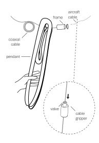
Push the valve on the cable gripper and adjust the position of the cable gripper so that the aircraft cable is roughly the same length as the coaxial cable.
