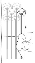
Very carefully uncoil the braided coaxial cable in a spool like manner. Insert your index fingers into opposite sides of the roll then rotate your fingers around each other to unroll the coaxial cable.
