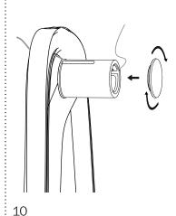
Screw frame cap back onto the frame assembly.
