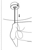
Very carefully uncoil the braided coaxial cable in a spool like manner. Insert your index fingers into opposite sides of the roll then rotate your fingers around each other to unroll the coaxial cable.
