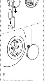
Plug the lamp into lamp socket. Check that each lamp is working properly as you go along. Slide the slotted cap through the cable and push down to
