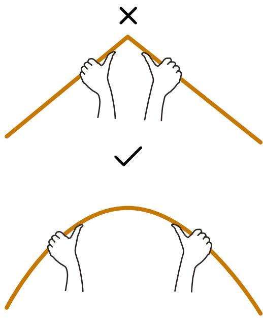
**EN** Very carefully uncoil the copper tube with both hands to avoid kinking. Be very careful not to overbend the copper tubes as it will leave a permanent kink that can not be removed.
