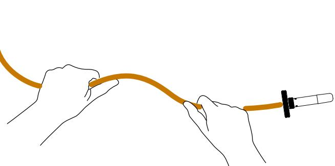
**EN** Compose the copper tubing according to the intended design aesthetic. Note: Once the pendant is added, it will pull the copper downwards. The pendant will try to hang directly below the canopy as the copper is not rigid enough for long horizontal compositions without the addition of pendant anchor kits.
