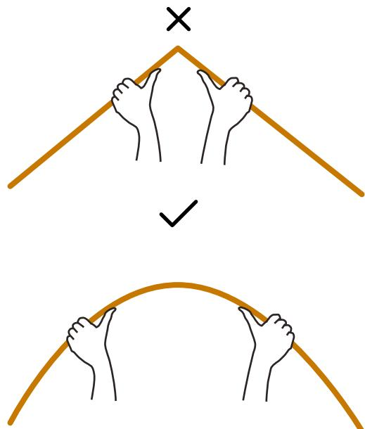
**EN** Very carefully uncoil the copper tube with both hands to avoid kinking. Be very careful not to overbend the copper tubes as it will leave a permanent kink that can not be removed.
