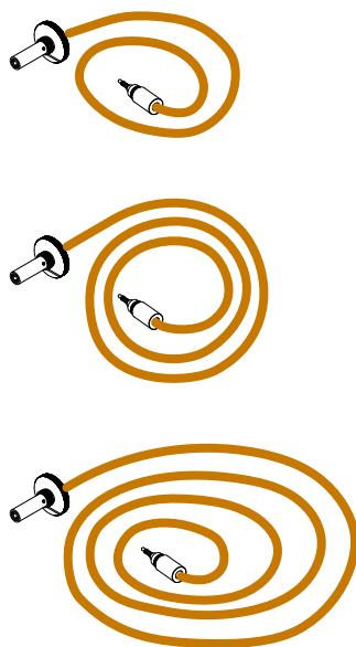
**EN** Separate the copper tubes according to length. Each copper tube is labeled with a series of numbers that correspond to its length in millimeters.
