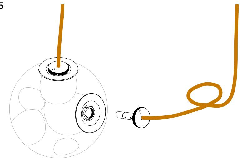
**EN** Gently form a loop with the tube approximately 130mm in diameter in the location of your choice. Insert the vessel into the loop and tighten the loop around the vessel, using the glass lip as a guide.
