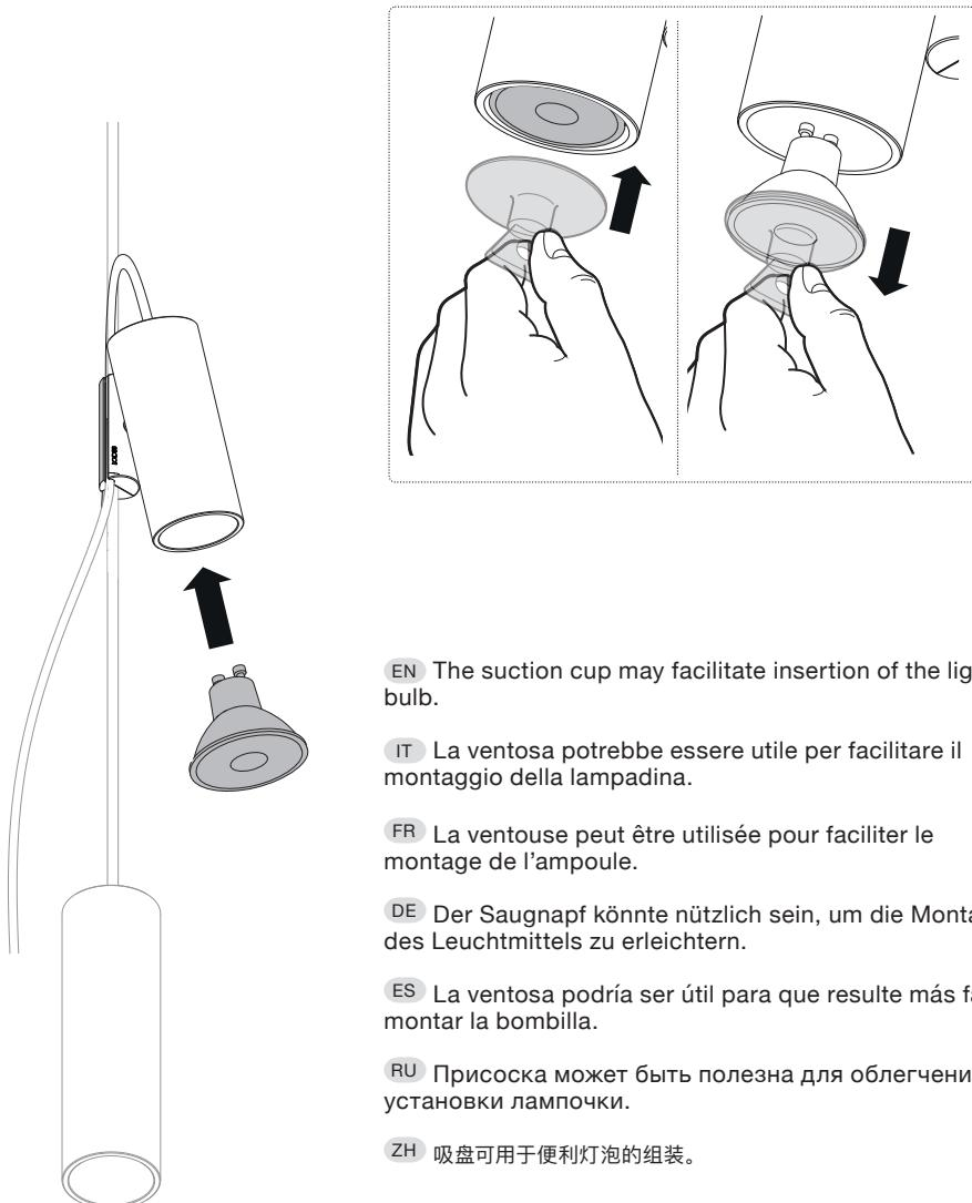
**EN** The suction cup may facilitate insertion of the light bulb.
