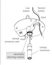
Feed the canopy connector wires through the slots on the canopy bracket. Attach canopy connector to the canopy bracket with a single screw, just to hold it in place.
