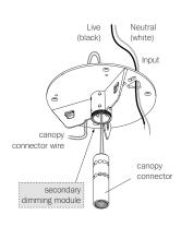
Feed the canopy connector wires through the slots on the canopy bracket. Attach canopy connector to the canopy bracket with a single screw, just to hold it in place.
