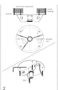
Measure and mark fixture location on the ceiling. Ensure the ceiling in this location has adequate structural support for the canopy bracket. Wood backing at least 3/4" (19mm) thick is recommended.
