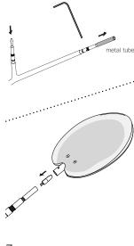
Remove the metal tubes at the end of each branch by unscrewing the set screw. Insert provided LED into socket. Check that each lamp is working properly as you go along by keeping the power on.
