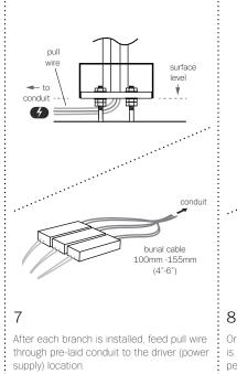
Connect burial cables to drivers (power supplies), ensuring to leave 100-155mm (4-6") of loose excess burial cable.
