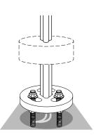
installing flush with the cover plate.
